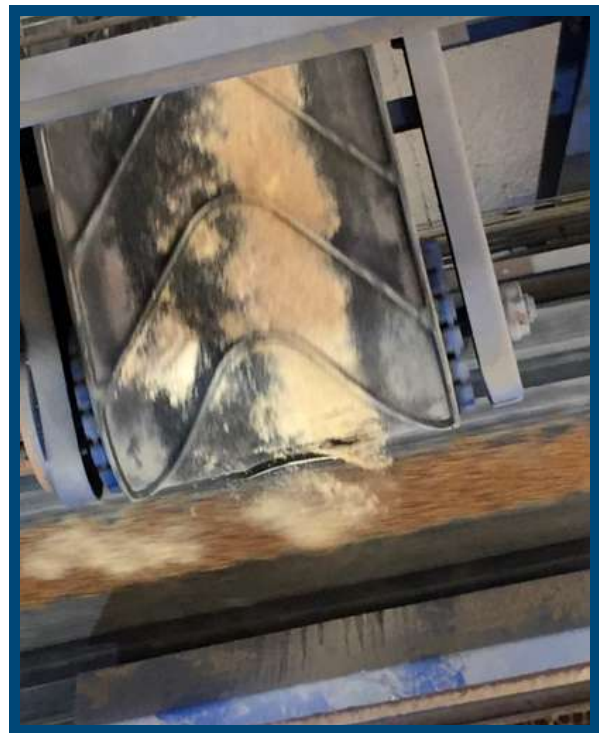
Separated substrate, before discharging the live and dead insects on the belt.
